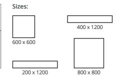
For a Raised Installation: Required pedestal positions based on size.
